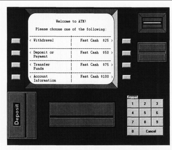
Figure 1. Illustration of the first screen of automatic teller machine simulator version 1 (ATM1). This simulator was modeled after an existing ATM. The background screen was gray and the menu options text was green.
