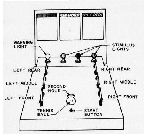
Figure 1. Diagram showing the apparatus used in the experiment form the perspective of the subject.
