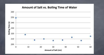
From this graph relating the amount of salt in the sample to the time it takes to boil, it can be seen that find the control (the sample containing no salt) to the first addition of salt, there is a significant drop in the time it takes to boil. The control took 249 seconds to boil while the sample with 7.5 ml of <sup>10</sup> salt takes 218 seconds, a drop of 31 seconds. From there, the graph also shows that the amount of time remains in the 218 range, and does not go above the initial drop.
