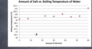
When relating the amount of salt to boiling temperature, the general trend is that an increase in the amount of salt leads to an increase in the boiling temperature. The control with no salt boils at 99.2°C, while the sample containing 60 ml of salt boils at 101.8°C, a total boiling temperature increase of 2.6°C. The sample with 15 ml of salt showed an unusual drop in temperature to 96.55°C, and has therefore been neglected; this can be attributed to experimental error.
