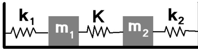
Figure 2: Coupled spring mass system with two masses.
